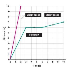
Bottom left is a distance-time graph. The gradient of the line is equal to the speed. This means that the line is: horizontal for a stationary object (because the distance stays the same); a straight diagonal for an object moving at a constant speed.
